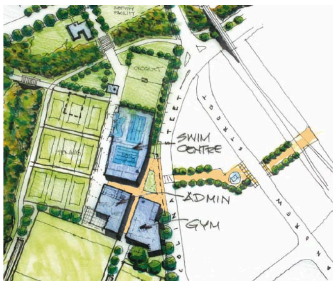
Detail of Plan for Sports Centre Complex, arranged to create a Plaza forecourt and pedestrian link to the CBD
