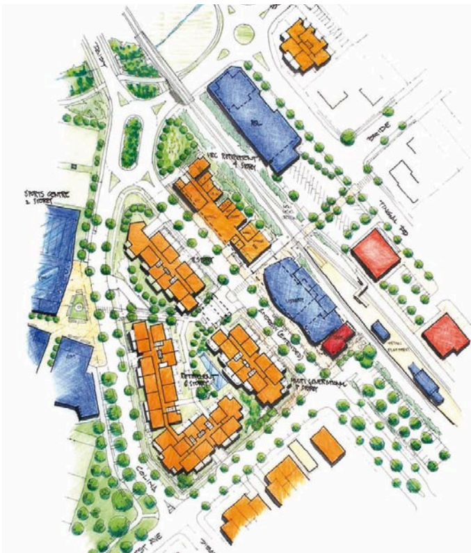
Station West Precinct Ground Floor Plan. Showing possible Library site in blue just next to the station, and various types of housing shown in orange, all facing out onto streets.
